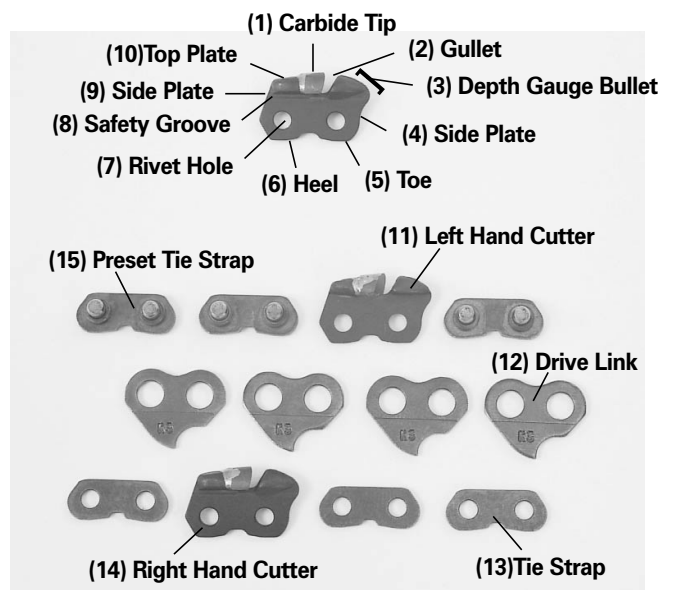
Fig. 26. Components of the BULLET® CHAIN
