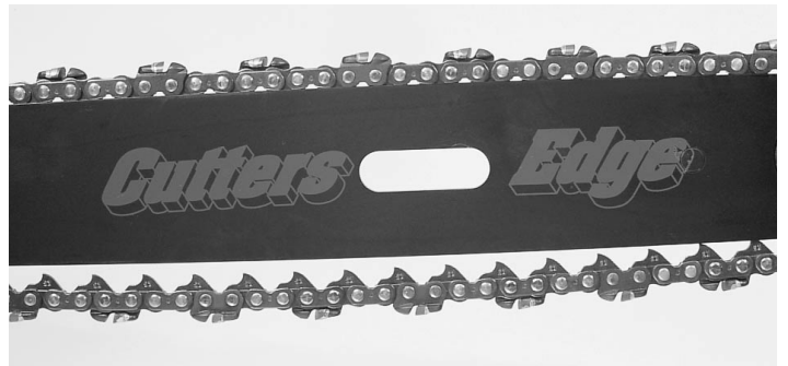
Fig. 9 "Sag" chain is too loose
