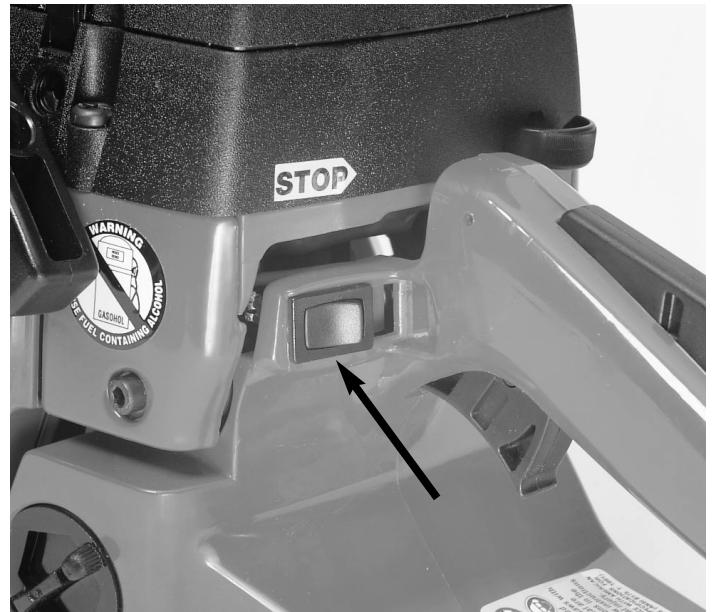
Fig. 12. Momentary Contact Switch
