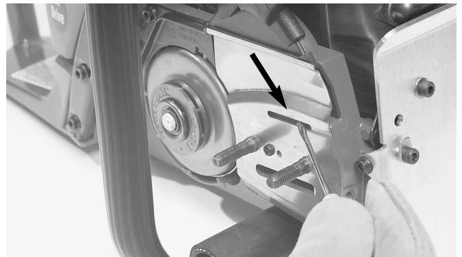
Fig. 32. Carefully clean out the oil slot
